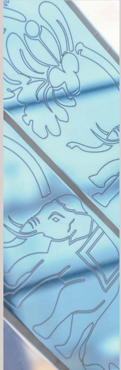
Semi-transparent OPV module with freeform print
